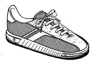
The finest in women's performance tennis shoes. The Whirlwind features a double durometer polyurethane outsole assembly. This consists of a cushioning layer of midsole urethane injected over a more durable urethane outsole layer. The V-throat all nylon mesh upper with foam padded collar looks as cool as it feels. The insole is an exclusive combination of supportive Ensolite® shock absorbent padding and polyurethane foam for a super soft feel, but cushioning as well. Made in U.S.A.
